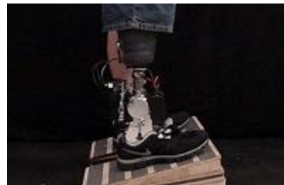
A robotic prosthesis for transtibial amputees
